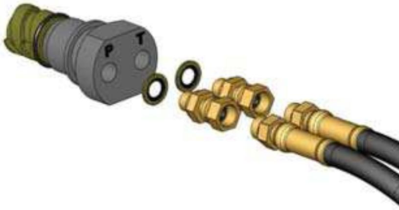
The male Mono Coupler must be installed on the tool connection hoses that are attached to a tool (Spreader, Cutter, Ram, etc.)
